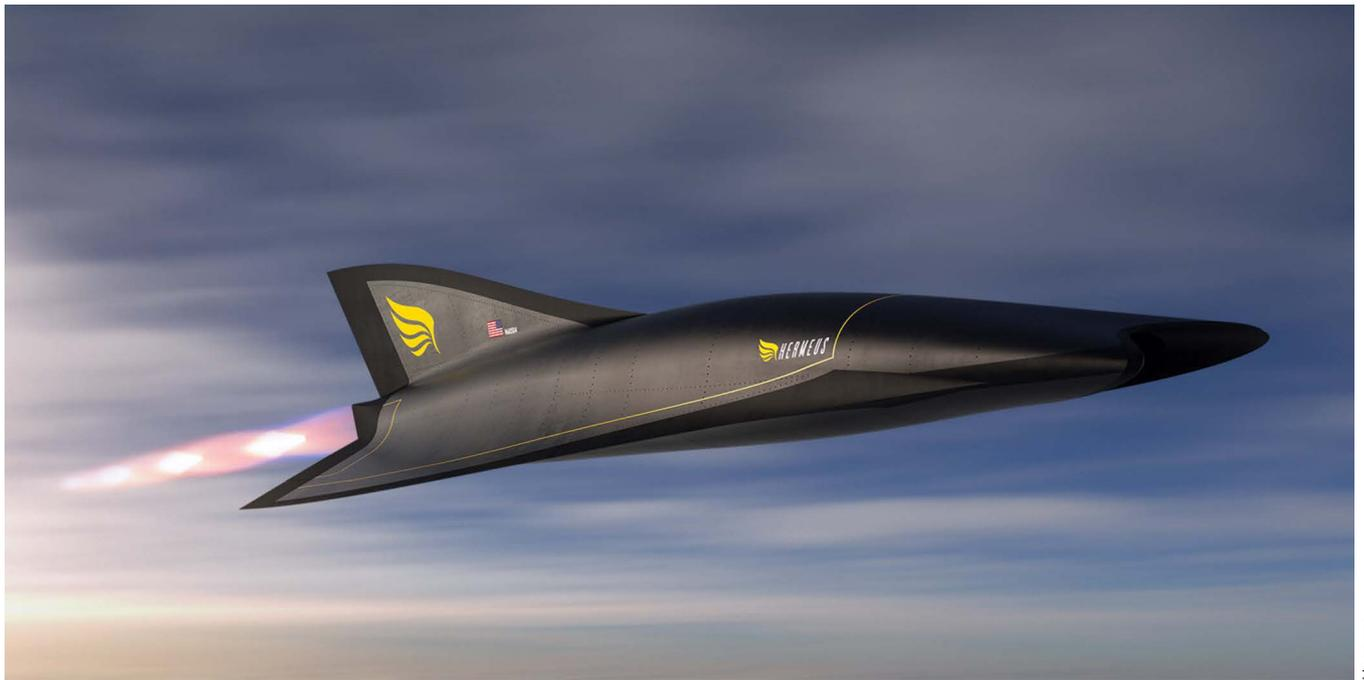
**Air Force testers will manage tests for the Hermeus Quarterhorse, shown here in a concept illustration, which is to be capable of flying at Mach 4. Quarterhorse will validate the company's proprietary turbine-based combined cycle (TBCC) engine, based on the GE J85 turbojet.**
