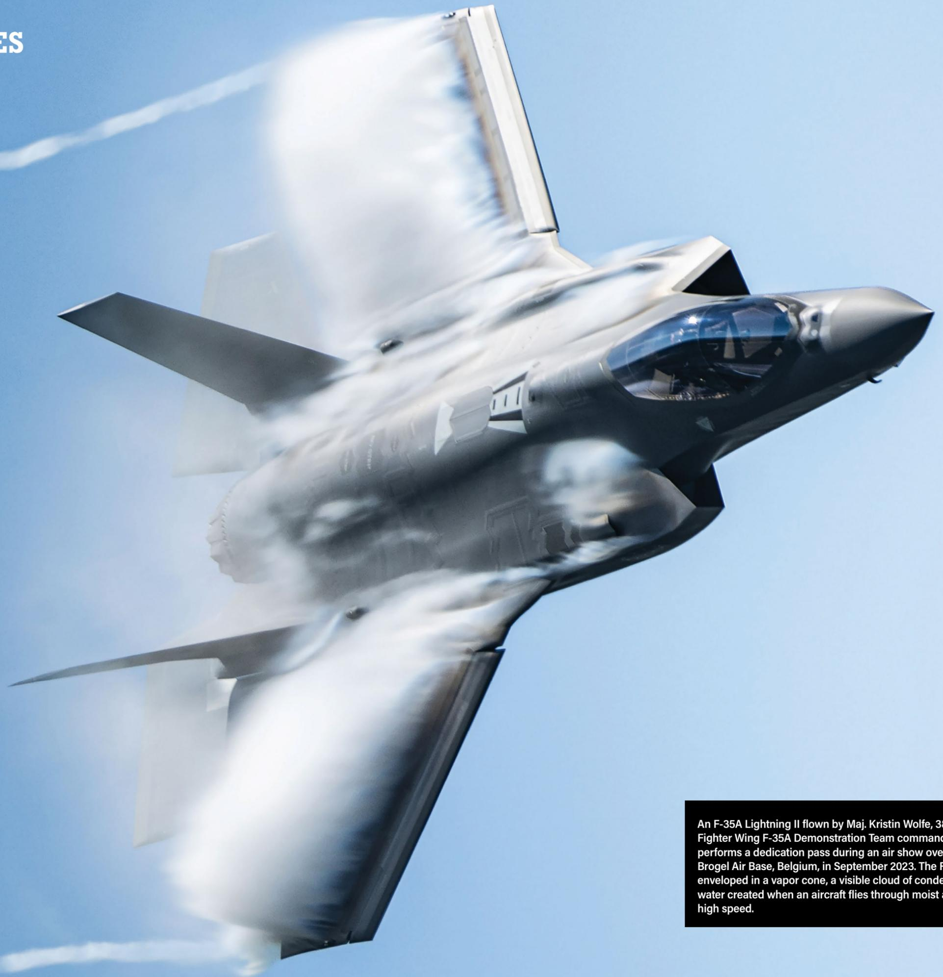
An F-35A Lightning II flown by Maj. Kristin Wolfe, 388th Fighter Wing F-35A Demonstration Team commander, performs a dedication pass during an air show over Kleine Brogel Air Base, Belgium, in September 2023. The F-35 is enveloped in a vapor cone, a visible cloud of condensed water created when an aircraft flies through moist air at high speed.
